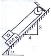
b) Determine the resultant of the given force system as shown in fig.
